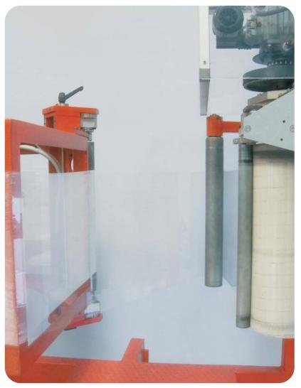
A top-rate adhesive polyethylene stretch film is obtained by a simultaneous extrusion process of four different prelaminated layers. Designed for palletizing loads of any kind, it can be used on fully automatic power-stretch machines up to 220% for the FPS, and up to 280% for the 18K. It comes also with an anti-UV treatment to resolve problems which may arise with loads stored out door.
