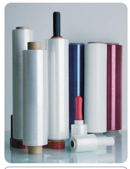
Deriblok is the only company to have the most varied and complete range of stretch film for manual use. Supplied with or without a dispenser, with an inner core which has been standardized to international formats 50 mm. (2 inch.) and 75mm. (3 inch.) it is an adhesive stretch film produced by the merging of four different layers during the extrusion process. This stretch film has been produced for all types of unusual packaging and/or limited spaces.
